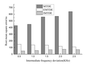
Fig. 5. Root mean square error versus intermediate frequency deviation,  $6\,\rm kHz$  wide signal band
