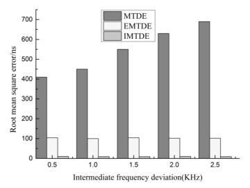
Fig. 4. Root mean square error versus intermediate frequency deviation, 8 kHz wide signal band
