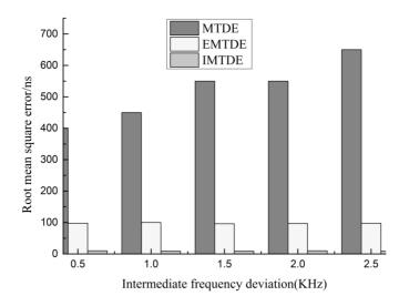
Fig. 3. Root mean square error versus intermediate frequency deviation,  $10\,\rm kHz$  wide signal band
