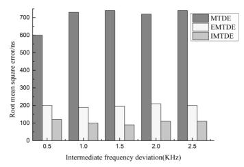
Fig. 6. Root mean square error versus intermediate frequency deviation, 4 kHz wide signal band
